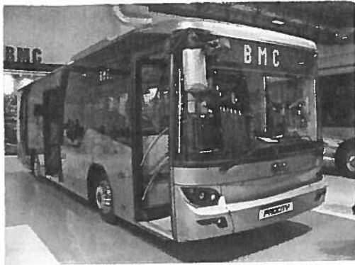
One of two prototype 10.05m long BMC Procity low floor buses shown by the reformed BMC business. This was to a city bus specification.
