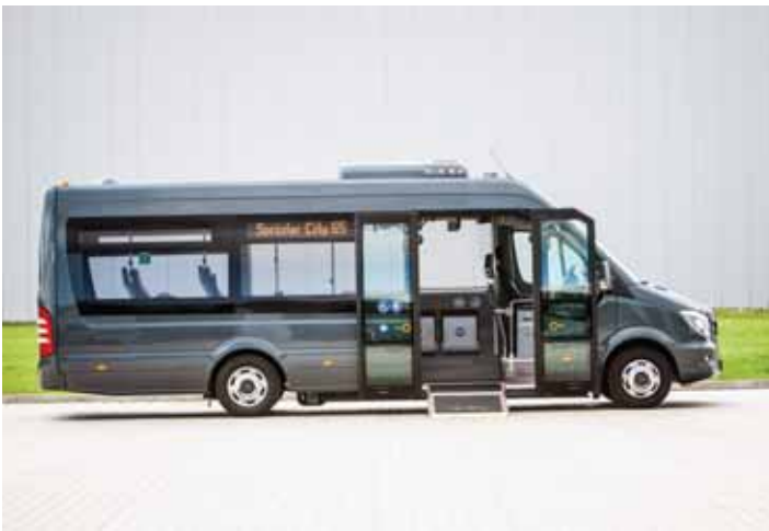
Although built on the Sprinter van platform, the Sprinter City 65 was obviously configured for city transit operation and could seat 13 passengers. OREN KIPNIS.
