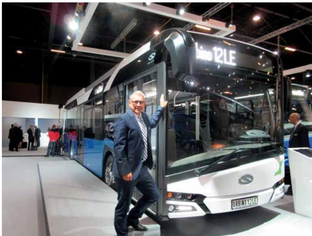
and significantly lighter in weight than its predecessor. Featuring a redesigned body frame with more passenger capacity, the Urbino 12 LE comes with a unified exterior, which allows operators to use many identical components and spare parts for different models of Urbino,
