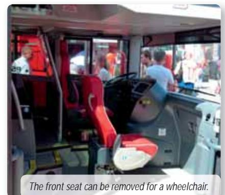
The front seat can be removed for a wheelchair.
