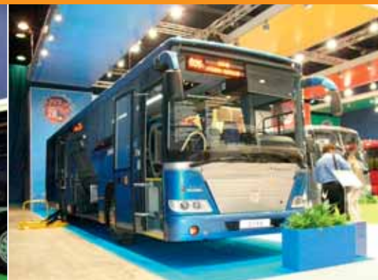
An interurban coach with a GoAZ body on a Scania chassis.
