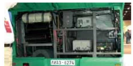
The electrical equipment on the LiAZ bus was in a full height compartment at the rear.
