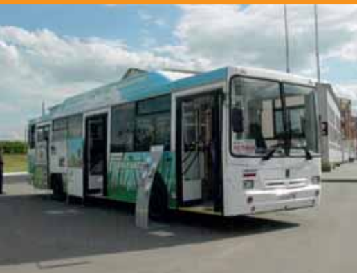
A NefAZ city bus fuelled by compressed natural gas.
