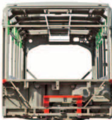
*The structure showing reinforcement beneath the driver and the roof meeting rollover regulations.*
