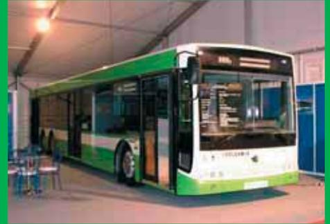
and to make new contacts. The City Rhythm has an Alcan aluminium structure and uses a number of Western European components in its driveline.
