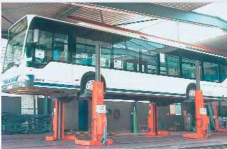
platform. Between the scissors there is absolute free access to walk underneath the platform and work beneath a vehicle.
