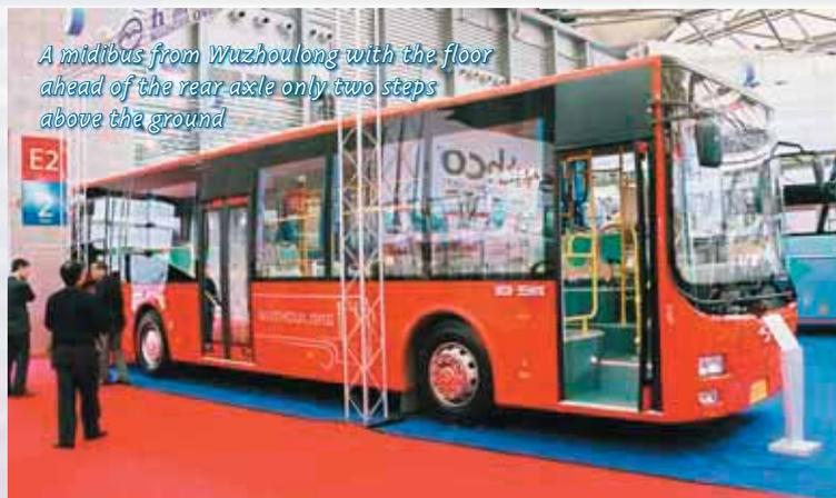
*A midibus from Wuzhoulong with the floor ahead of the rear axle only two steps above the ground*
