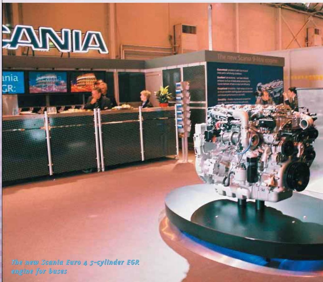
*The new Scania Euro 4 5-cylinder EGR engine for buses*
